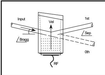
The D110-T50S provides high speed laser beam scanning and each model is optimized for a specific operating wavelength in the NIR spectrum. The D110-T50S may be operated in raster (linear), random access and vector scanning modes from the same RF drive electronics. The Isomet deflector-driver combination is designed to maintain the Bragg relationship over the specified RF frequency bandwidth. This results in a uniform diffracted beam intensity across the full scan angle.
